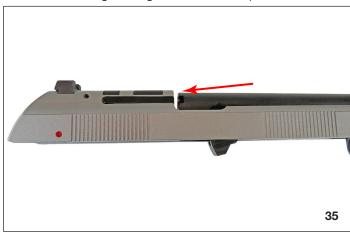
The recoil spring guide head should lodge in the center of its groove in the locking block.
