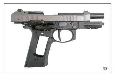
Slide the back strap grip over the rear of the lower receiver.
