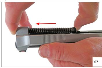
Lift the spring guide and recoil spring, letting the spring out slowly, as it is under tension.
