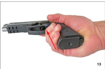
Grasping the slide serrations with thumb and index finger, fully retract and release the slide to load the chamber.
