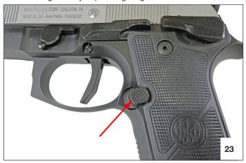
Press and hold the disassembly lever release button.
