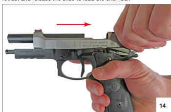
**(SAO Only)** Once the chamber is loaded, press the safety lever up into the safe position until ready to fire.
