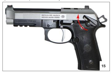
**(DA/SA Only)** Once the chamber is loaded, rotate the de-cocker lever up to safely drop the hammer to half-cocked position.
