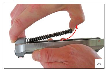
Remove the barrel and locking block assembly from slide.
