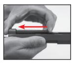
Lift spring guide and recoil spring, letting the spring out slowly, as it is under tension. (figure below)
