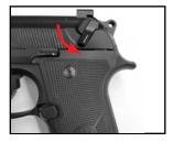
Depress the magazine release catch to remove the magazine from the pistol. (figure below)  $\,$
