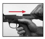
Once sure that the chamber is empty, and the cartridge has been ejected, release the slide.
