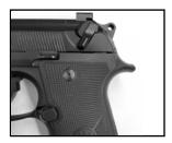
The barrel should rest perfectly flush against the slide (the extractor must rest in its groove in the barrel). (figure below)
