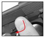
Pull the slide assembly forward. (figure below)
