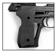
Reinstall the grip screws and lock washers with a 2MM Allen wrench by turning them clockwise. (torque to 10 inch pounds) (figure below)
