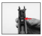
When rotating the disassembly lever, the slide should be in the closed position (aligned with or beyond the rear side of frame).
