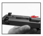
The recoil spring guide head should lodge in the center of its groove in the locking block.(figure below)
