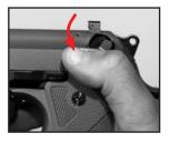
Depress the magazine release  $\,$  button to remove the magazine from the pistol. (figure below)
